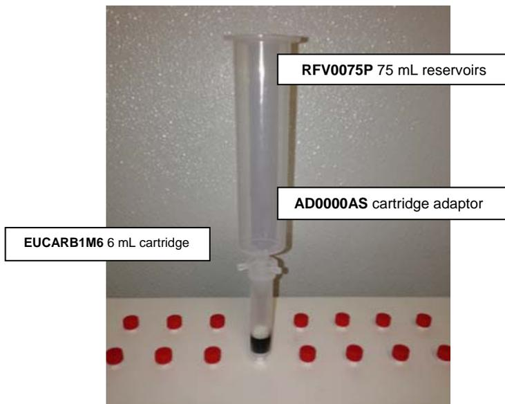
**Detail of Reservoir, Adaptor, and Cartridge Setup**
