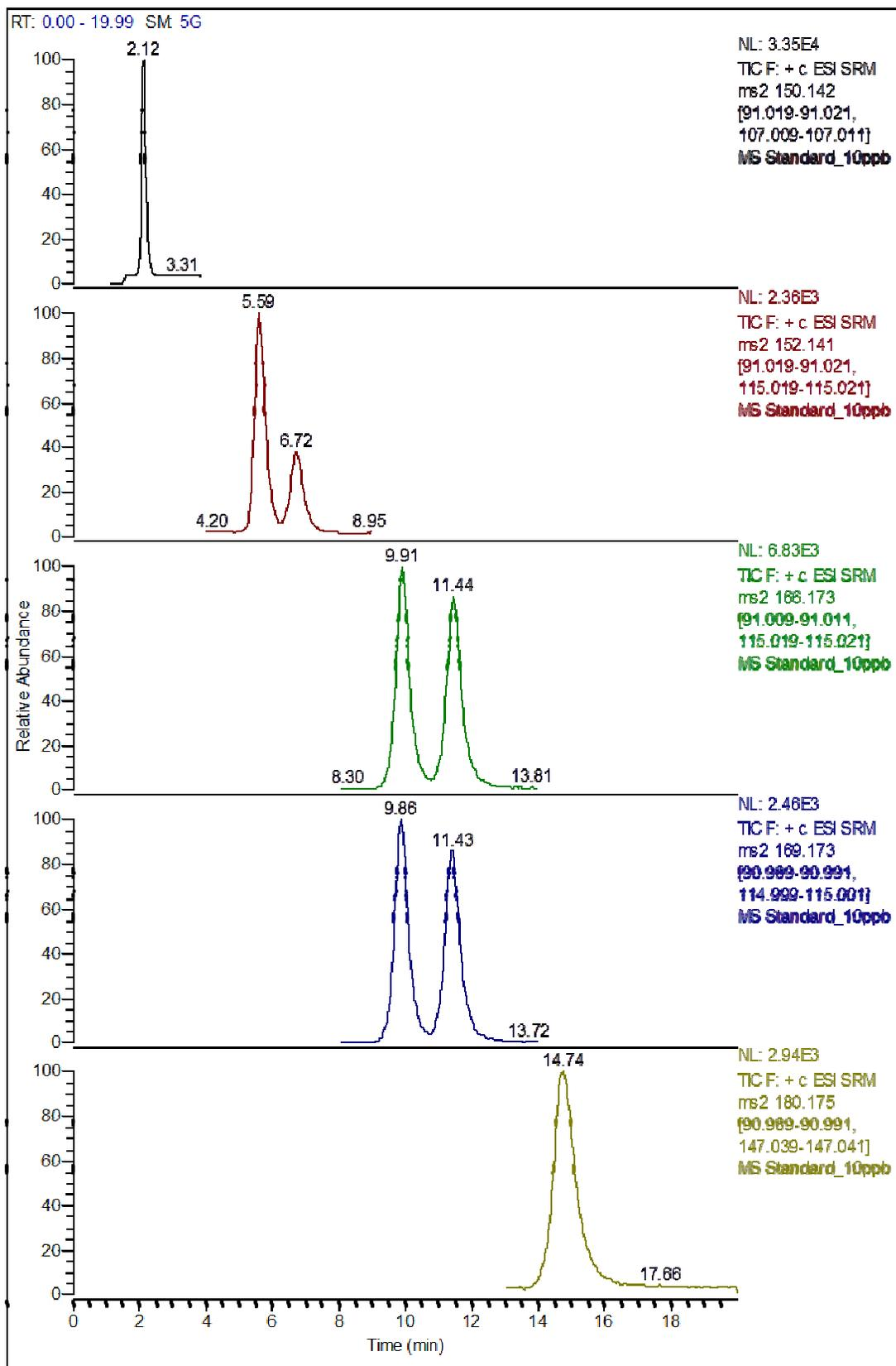
Figure 2. Chromatogram of a 10 ng/mL standard.
