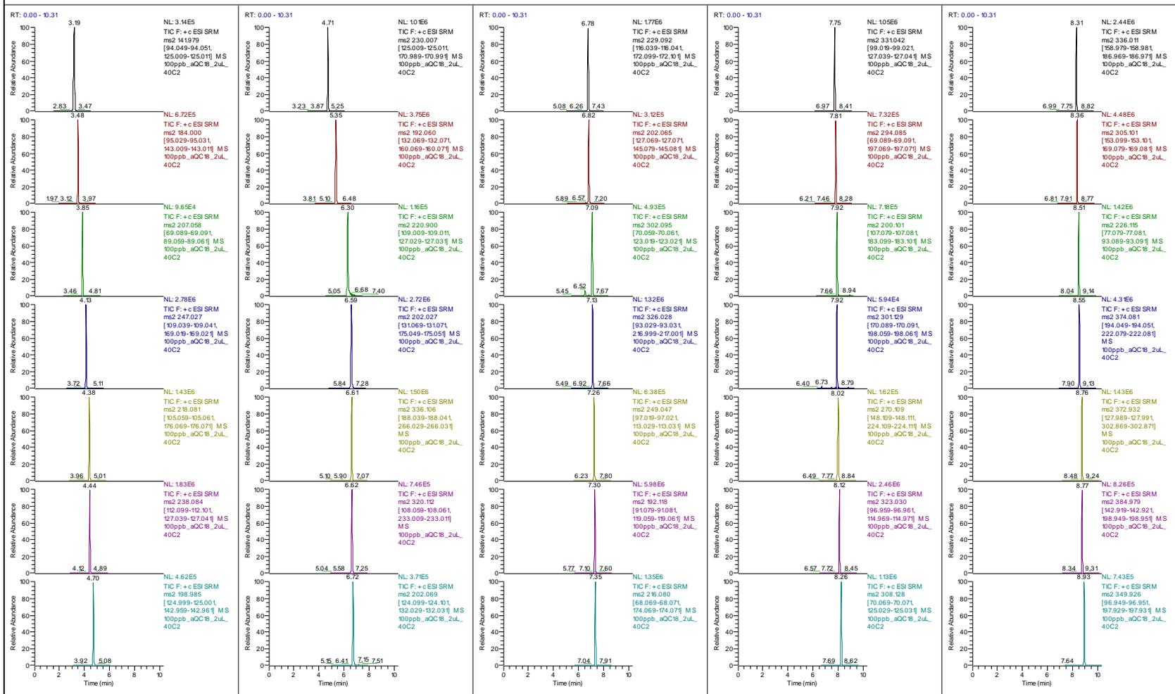
**Chromatograms of 34 Pesticides and TPP (IS) in 1:1 MeCN:H<sub>2</sub>O (100 ppb) using UCT Aqueous C18 HPLC Column (Compound order can be found in the SRM table.)**
