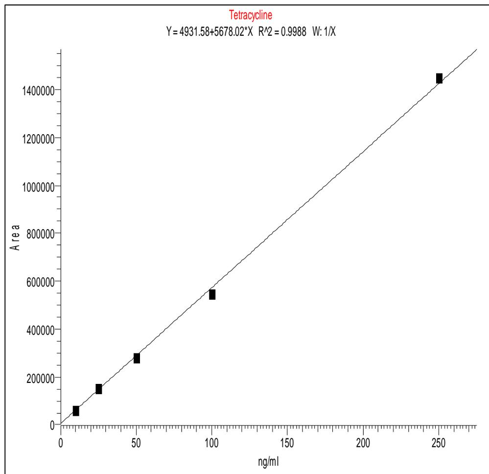
**Figure 3.** Calibration curve example (tetracycline).
