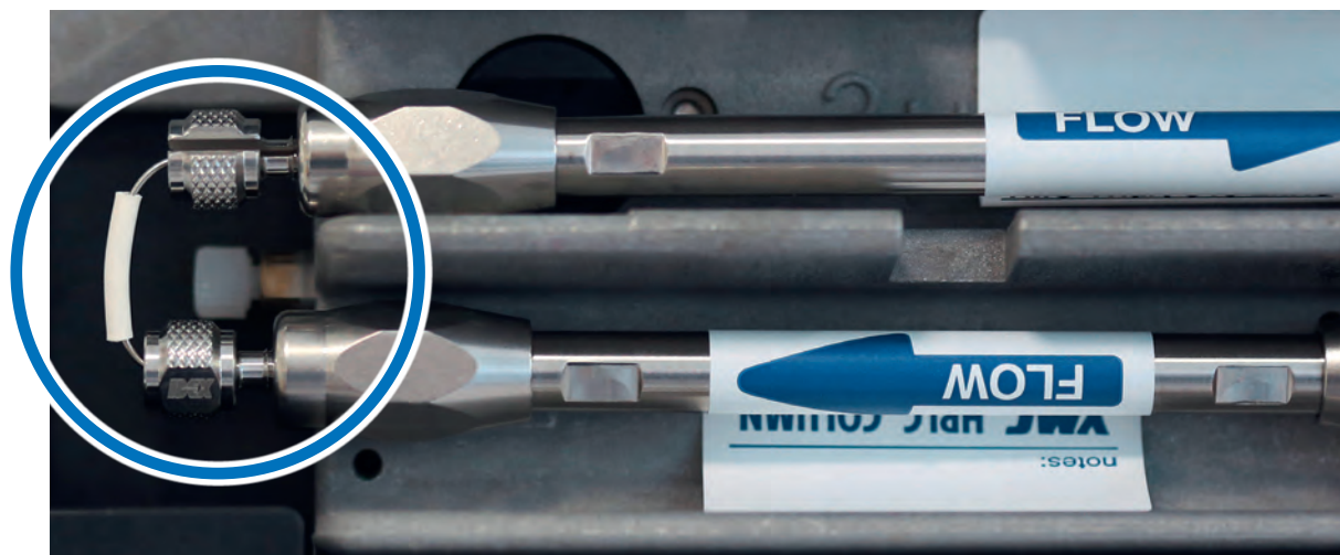
Coupling of two YMC-Triart UHPLC columns using the dead volume free MarvelX™ connector.
