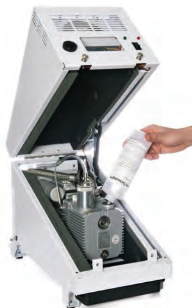
Quiet Cover GC/MS, with open-access cover
