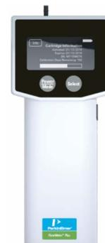
The PerkinElmer Flowmeter Plus is a valuable tool for troubleshooting detector problems. Measuring gas volumetrically eliminates the need to select gas type. Highly accurate, identifying leaks by differences in thermal conductivity, it offers a minimum detection limit of 0.0005 mL/min hydrogen and helium.
